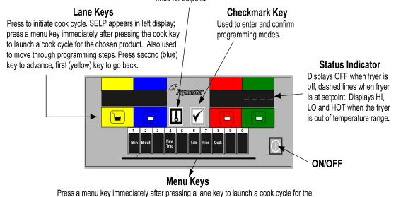
desired product. The keys are also used to enter names of products. Each button, when repeatedly pressed, accesses multiple letters or symbols. See example below.
